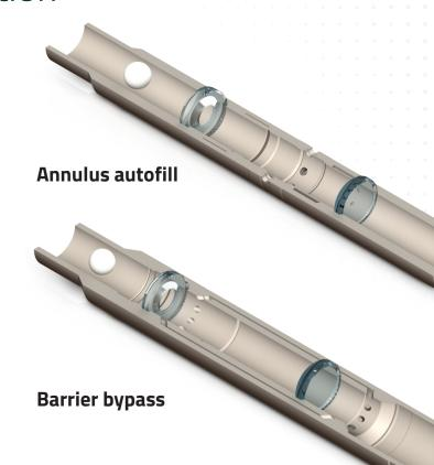
Combining the Fantom™ Shatter Ball Seat (SBS) and Barrier provides the perfect solution for autofill. To benefit from this combination, the valve is installed with the flow ports in an open position, which allows fluid from the annulus or below the plug to fill the tubing string. As a result, it improves well control during RIH and ensures a smoother deployment process.
